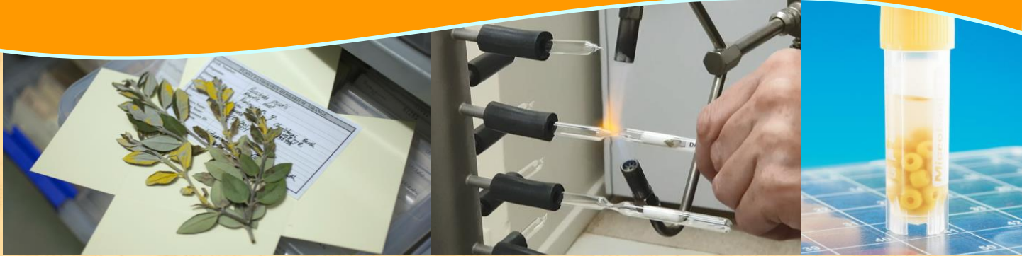
Fig. 1. a) Dried herbarium specimen of Myrtle rust b) Sealing a glass ampoule c) The microbank bead system
